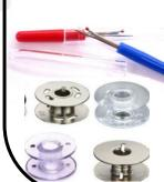
A seam ripper is a small tool used for unpicking stitches.
